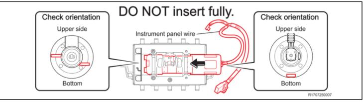
b) Connect the airbag connector to the instrument panel passenger airbag assembly and then push in the airbag connector lock as shown in the illustration.
