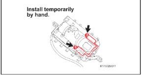
Temporarily install a NEW plate and airbag inflator with the 2 NEW self-locking nuts.
