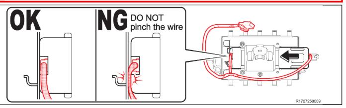
Insert the inflator with the correct orientation as shown in the illustration.
