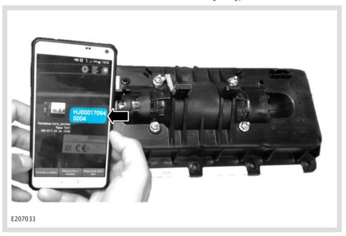
Use a smartphone with a QR scanner application to scan the QR code on the passenger airbag module label.
