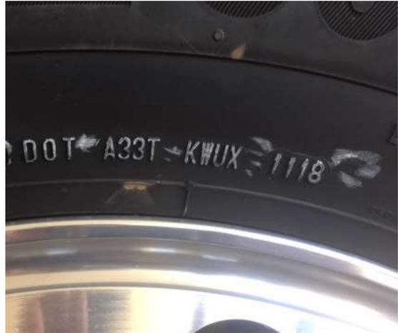
Tires made for use in the United States are required to have the DOT serial number and date located on one sidewall of the tire near the rim. The sample shows a tire manufactured during the 11<sup>th</sup> week of 2018.
