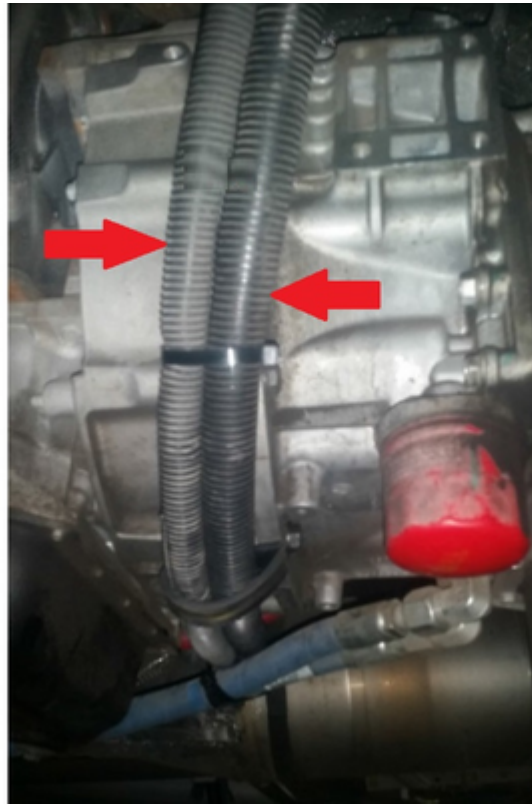
Figure 11, New Refrigerant Hose Routing.
