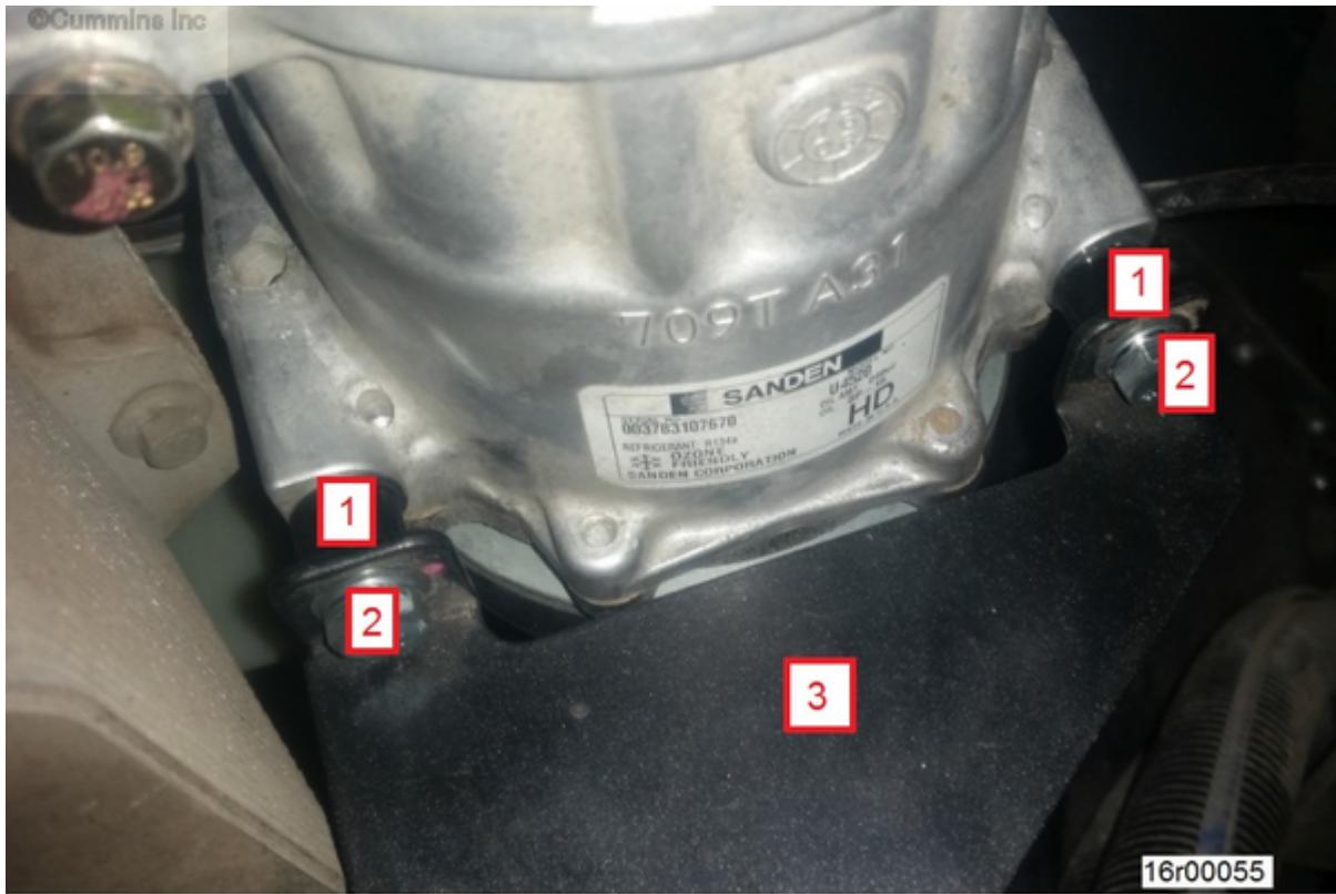
Figure 5, New OEM Bracket, Part Number 5073826. Top View.
