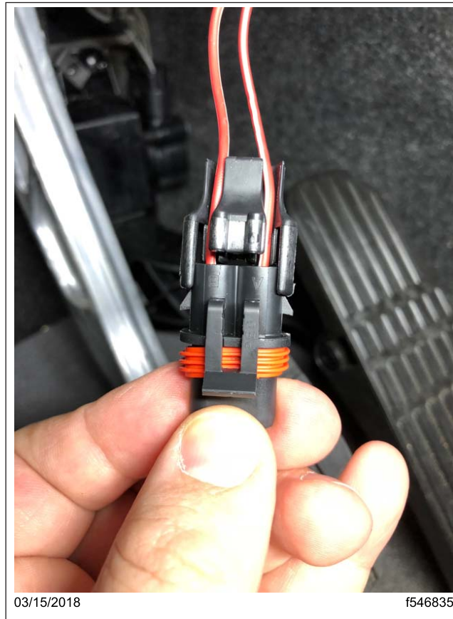
Fig. 6, Switch Connector, Back Cover Partially Removed
