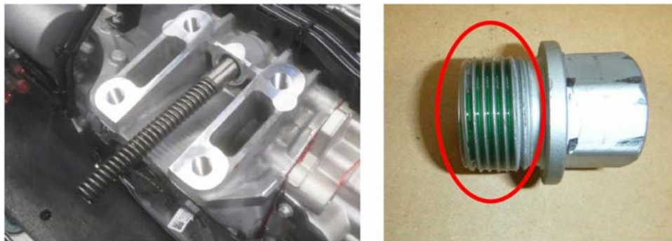
Figure 4 – Installation of Range Shift Fork Detent Spring Nut Cap
