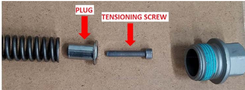
Figure 3 – Removal of Plug and Tensioning Screw
