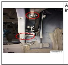
A. Visually check if all components are contacting without space in between.
