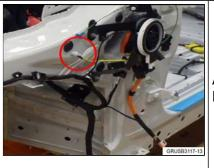
A. Ground point of charging receptacle needs to be torqued to 8 Nm thru wheel housing.
