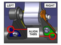
• Tighten the tie rod nut to 44 N•m (4.5kgf•m, 32 ft•lb).
