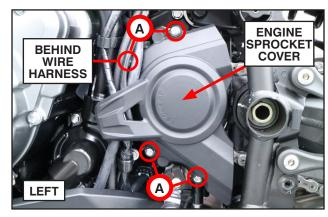
• Tighten the middle rear engine mounting nut [A] and lower rear engine mounting nut [B] to 44 N•m (4.5 kgf•m, 32 ft•lb).
