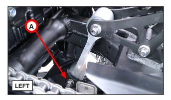
Raise the rear of the frame slightly with suitable straps [A] passed through the rear footpeg brackets [B] to unload the weight on the rear suspension in order to remove the bolt easily.
