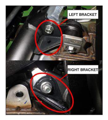
Position the special left washer from the repair kit along the bottom of the frame bracket as shown.
