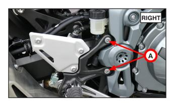
• Loosen the tie rod nut [A] but do not remove it at this time.
