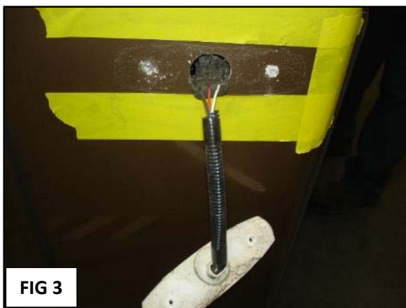
FIG 3: Remove light from the vehicle, and pull the harness plug out through the hole. Harness plug should still be sticking out of the hole in the vehicle.
