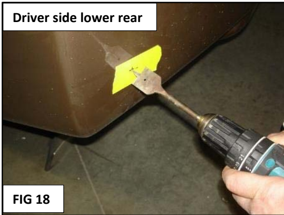
FIG 18: Use the drill with the 1-1/4" drill bit. Drill the two holes at the rear driver and passenger locations.
