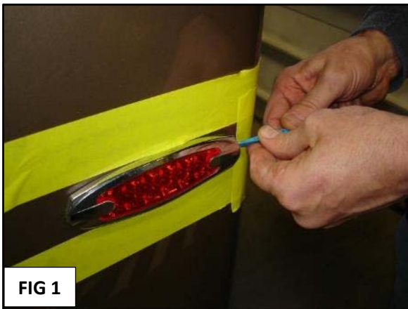
FIG 1: Tape around the existing marker light as a guide for placement of new light. Gently pry off the chrome bezel using the plastic putty tool and a flat screwdriver. There are four tabs under the bezel holding it to the light base.
