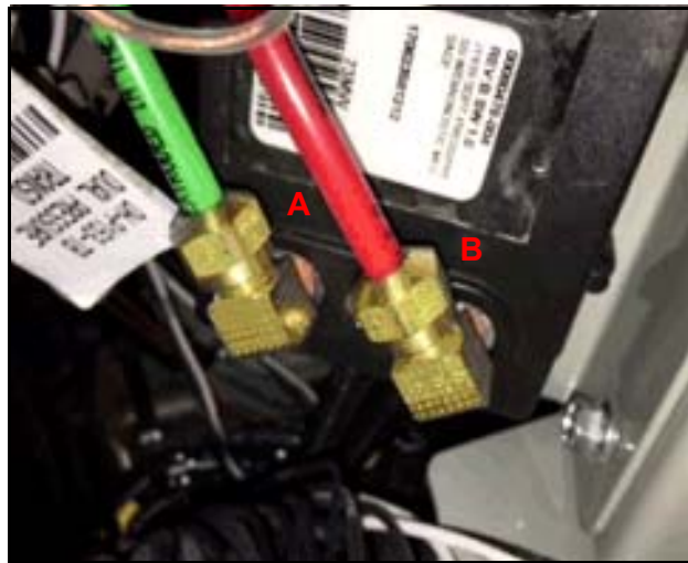
Figure 4. Routed air line connection to brass, 90 degree elbow.
