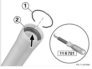
• **Pad** a suitable leverage tool, e.g. slide a suitable petrol hose **(1)** onto the lever (11 6 721).
