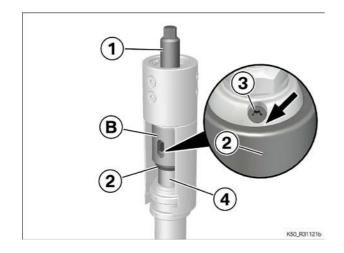
• Using the spindle (1) and the thrust piece (B) press-fit the fixed fork tube bushing (2) to the limit position or with tightening torque.
