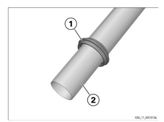
• Slightly lubricate the inner face of dust boot (1).
