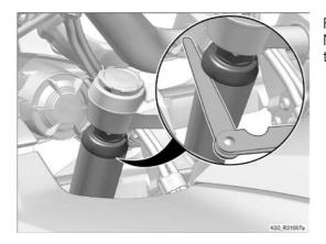
Figure 1: seal plug of the fixed fork tube (stanchion) Note: for the inspection, the rubber grommet (not pictured) mounted at this location must be pushed down to view and measure any gaps.
