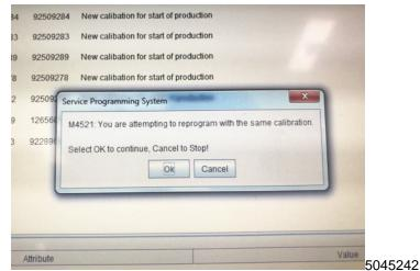
Note: If the Same Calibration/Software Warning is noted on the SPS controller screen, select "Ok" and continue programming.
