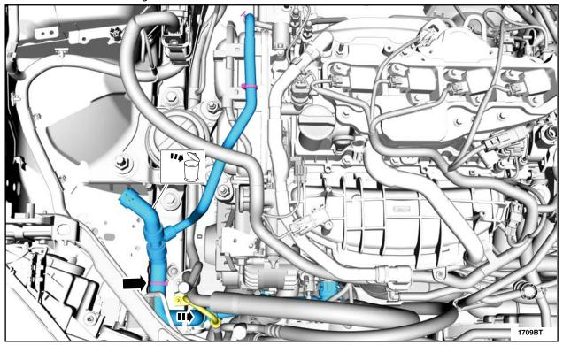
6. Detach the retaining clip and disconnect the degas bottle hose from the engine oil cooler assembly. Remove and discard the degas hose assembly. See Figure I7.
