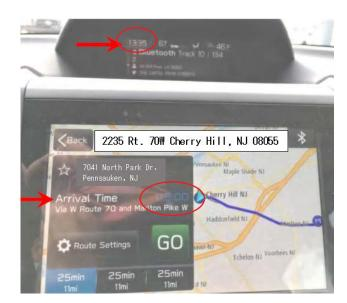
2) Time of day displayed in the MFD (Multi-Function Display) is incorrect and the arrival time displayed in Navigation units is also incorrect.
