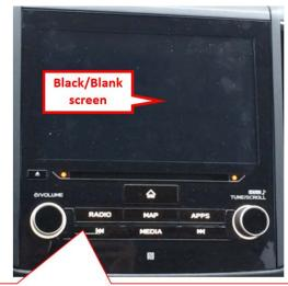
Hard key (button) illuminated, on solid or flashing / blinking
