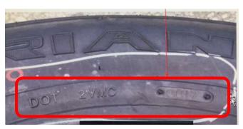
The DOT code is located under the word "Triangle". Tires covered by this recall will have DOT codes **2VMC 0517** or **2VMC 0617**.
