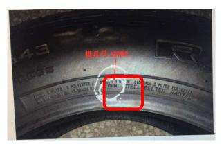
The Mold Number is located between the pattern name TR643 and the word "Radial", near the bead. Tires covered by this recall will have Mold Number **13HM**.
