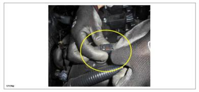
6. Unclip the two head cover clips on the left side.
