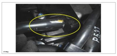
25. Install the oil dipstick in a vertical position.
