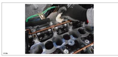
16. Remove the old hardened sealant and apply new sealant at the four points shown on the front cover (A), the
