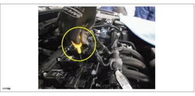
4. Disconnect the four ignition coil harness connectors.
