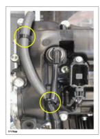
24. Connect the ventilation hose to the head cover, matching the hose mark with the groove.
