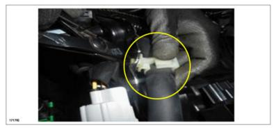
10. Remove the four ignition coils by removing the four bolts from left to right using an 8 mm socket.
