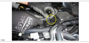
9. Disassemble the vacuum hose clip.
