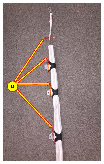
14. Install the new passenger and driver curtain airbag assemblies in the vehicle following the procedures detailed in the 2013-2018 Santa Fe Sport Service Manual (Restraint) section. Torque each nut and bolt to the spec shown below.
