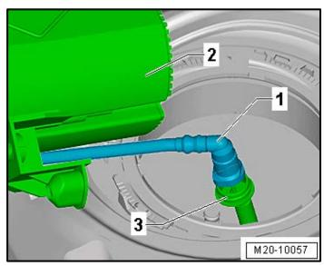
• Coat the inside of the new fuel delivery unit seal <1> with fuel and install into the opening in the fuel tank.
