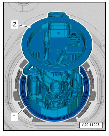
• Reinstall the fuel delivery unit, using caution not to bend the fuel level sensor when installing.
