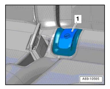
• Reinstall the covers <1> to the LATCH child seat anchors <arrow>.
