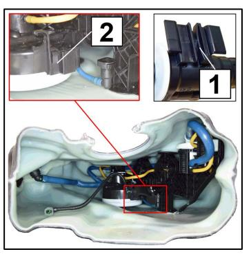
Release the retainer <3> and transfer the front • suction line <1> from the old suction pump <2> to the new suction pump, ensuring that the locking of the retention clip <3> is felt and/or heard.
