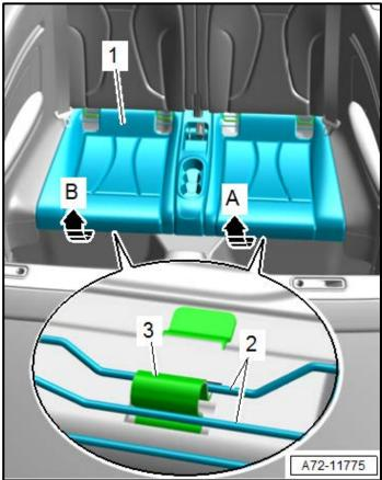
• Push the guides <1>, corresponding to cutout, downward and disengage them from the LATCH child seat anchors <2>.
