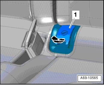
Unclip and remove the covers <1> from the LATCH child seat anchors <arrow>.
