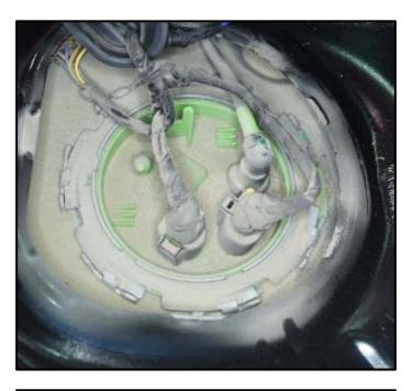
Prior to disassembly, the fuel delivery unit MUST be clean. If excessive dirt or debris is present <as shown>, clean and dry the fuel delivery unit and surrounding areas as necessary.
