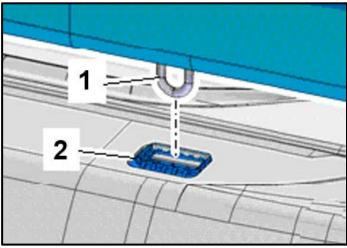
Install the rear bench seat and push the wire hooks <1> into the mounting grommets <2>.
