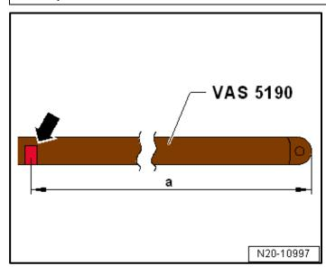
Use insulating tape to mark the hose <arrow> at the distance <a> from the end of the suction hose on the -VAS5190-.
