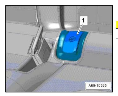
Reinstall the covers <1> to the LATCH child seat anchors.
