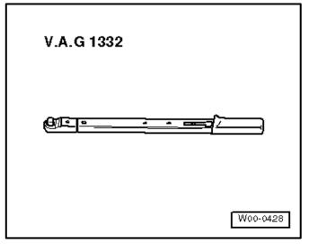
Torque Wrench 1332 40-200Nm -VAG1332- (or equivalent)
