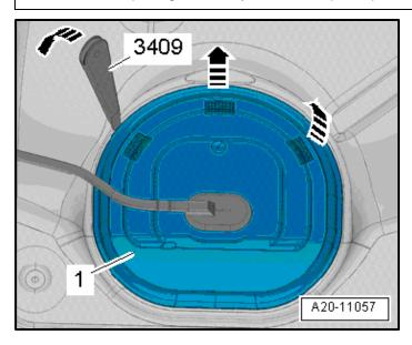
In the rear seat, unclip the sealing flange cover <1> at the tabs <arrows> using the Trim Removal Wedge -3409-.
