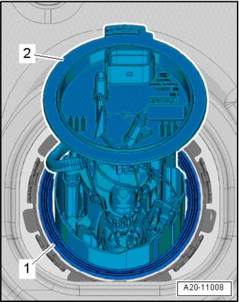
Carefully guide the fuel delivery unit with the fuel level sensor through the opening into the fuel tank.
