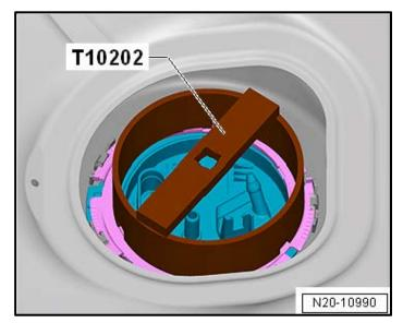
• Using the -T10202-, tighten the locking ring to 110 Nm.
