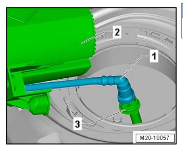
When reconnecting fuel lines, ensure that the locking of the retention clip is felt and/or heard.
