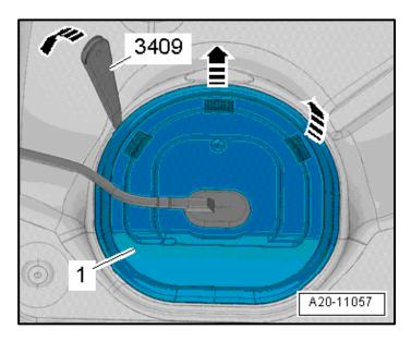
In the rear seat, unclip the sealing flange cover <1> at the tabs <arrows> using the Trim Removal Wedge -3409- (or equivalent).
