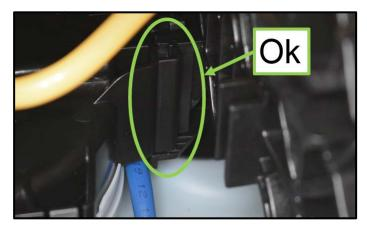
When correctly installed, the Liquid-Vapor Separator clip will be secured into its mounting bracket as shown.
