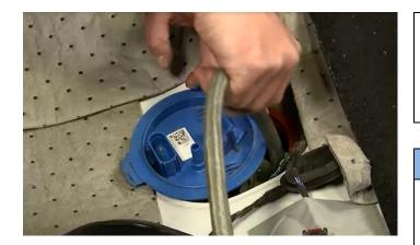
Use cold weather protective gear or equipment as necessary, drain all of the fuel out, or warm the vehicle indoors if the vehicle has been stored in an extreme climate condition before performing the next steps.
