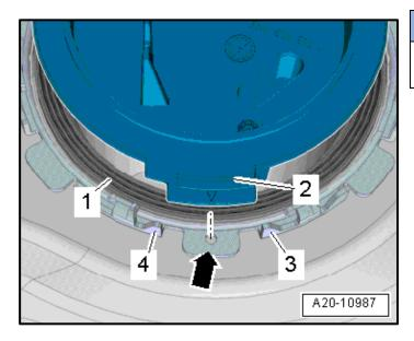
When inserting the sealing flange, the seal must not be damaged or crushed.
