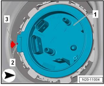
• The arrow <3> on the fuel tank must point to the mark <2> on the sealing flange <1>.
