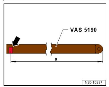
Use insulating tape to mark the hose <arrow> at the distance <a> from the end of the suction hose on the -VAS5190-.
