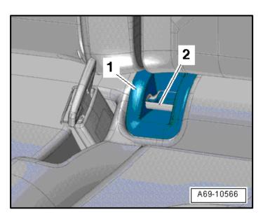
Reinstall the guides <1> to the LATCH child seat anchors <2>.
