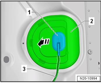
Unclip the grommet <1> downward out of the cover <2>.
