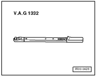
Torque Wrench 1332 40-200Nm -VAG1332- (or equivalent)
