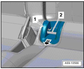
• Push the guides <1>, corresponding to cutout, downward and disengage them from the LATCH child seat anchors <2>.
