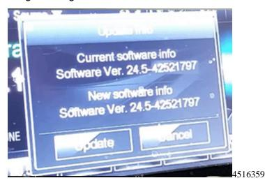
**Note:** When USB programming has completed, the radio will go to the Home/Menu screen, and the calibration ID screen will show, confirming the current and new software is now the same. Audio should be playing before removing the USB drive. Select "Cancel" and continue to step 10. (Trax shown as example-Sonic and Spark will be similar).
