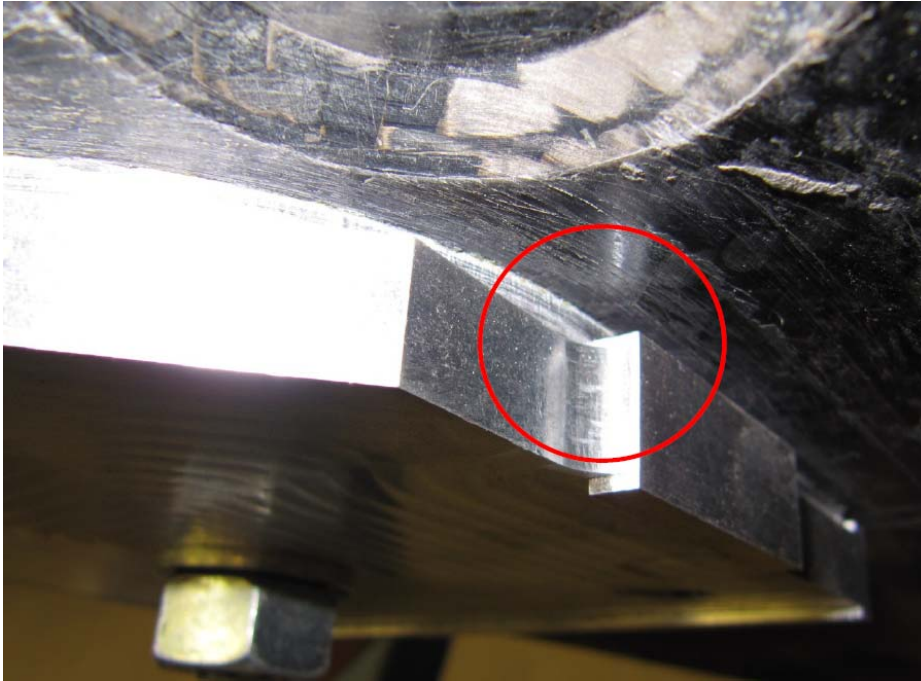
Fig 5: Installation position of the drilling gauge on the Monocoque with Detail Y stop
