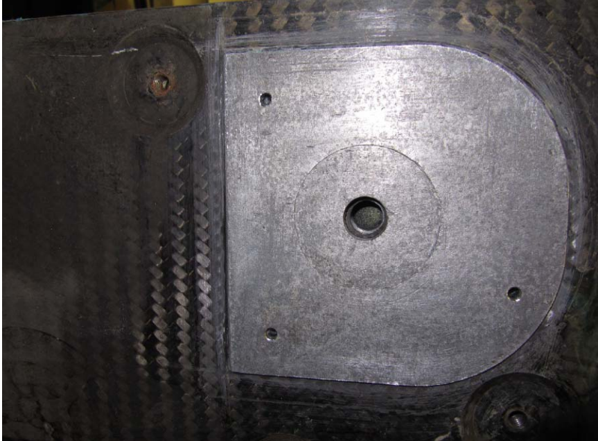
Fig 6: RPS-Plate with the 3 drilled and deburred holes (Ø5,0mm)
