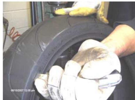
Measure 8-12 inches along the sidewall of the tire and then make a visible cut through sidewall of the tire that length. This method is described in the two photos above. Please use gloves and precaution when making the cut.
