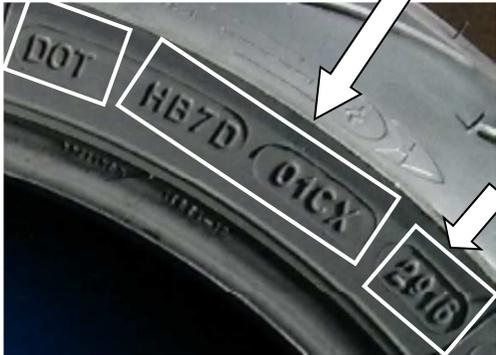
The example shows a date code of "2916", indicating "week 29 of 2016". The Tire Identification Date Code on the recalled tires is 1616, 1716 or 1816. If the tire has any Date Code other than the 3 listed above or is not a 180/55ZR17 M/C (73W) Pilot Power 3 tire, it is NOT affected by this Recall notice.
