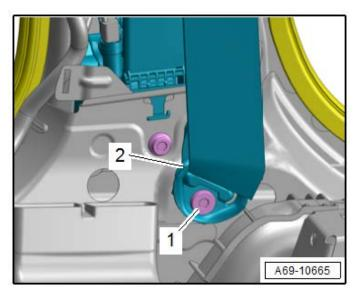
Install lower belt relay <2> and torque bolt <1> to 40 Nm.
