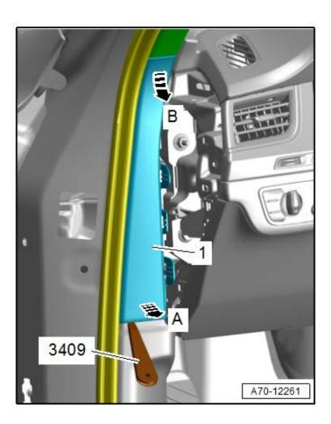
Unclip the A-pillar gap cover <1> using the -3409- <arrow A> and disengage at the A-pillar upper trim panel <arrow B>.
