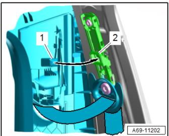
Guide the belt webbing and seat belt latch in through the slide for the seat belt height adjuster.
