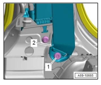
Remove the bolt <1> and then remove the belt relay <2>.
