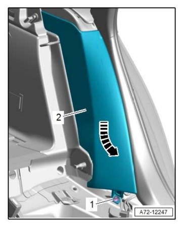
Install side cushion <2> and torque nut <1> to 9 Nm.
