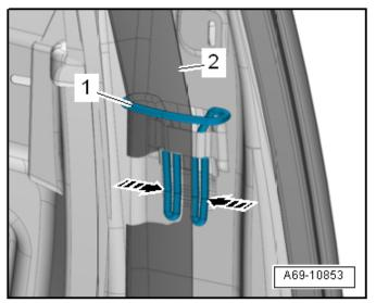
Push the bracket together <arrows> and remove the belt guide <1> upward.
