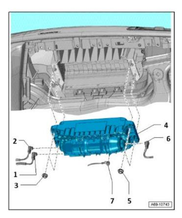
Install the new airbag unit <4> using new nuts
