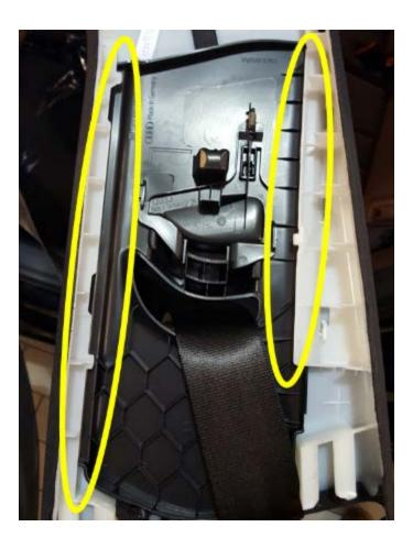
Before installing the upper B-pillar trim, ensure the seat belt height adjuster is installed correctly in the guide rails.
