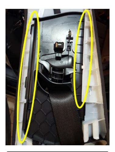
Before installing the upper B-pillar trim, ensure the seat belt height adjuster is installed correctly in the guide rails.
