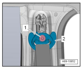
Install seat belt relay <2> and torque bolt <1> to 45 Nm.
