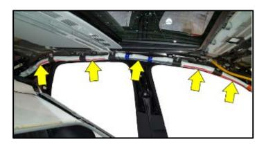
Unwrap the head curtain airbag, making sure the colored strips are visible along the entire length. This will ensure that the head curtain airbag is not twisted.
