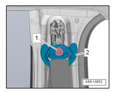
Install seat belt relay <2> and torque bolt <1> to 40 Nm.
