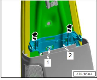
Release the catch <1> using a screwdriver and pull the bracket <2> for the B-pillar trim panel upward out of the mounts <arrows>.
