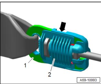
Open the cover <2> for the belt anchor <1> with a screwdriver on the catches <arrow>, open and push aside.
