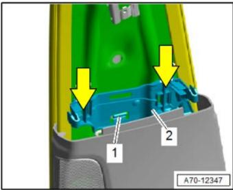
Slide the bracket <2> into the mounts in the direction of <arrows> until catch <1> audibly locks.
