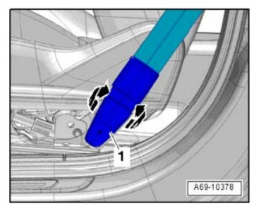
Install the belt end fitting over the pin on the seat frame and pull up on the belt end fitting until the lock audible engages.
