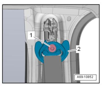
Install seat belt relay <2> and torque bolt <1> to 40 Nm.
