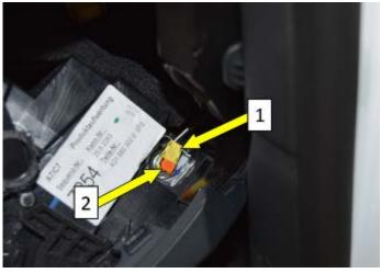
Connect knee airbag connector <1> and engage lock <2>.
