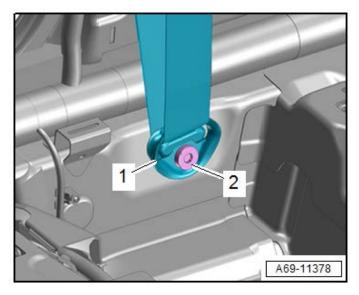
• Install bolt <2> and torque to 40 Nm.
