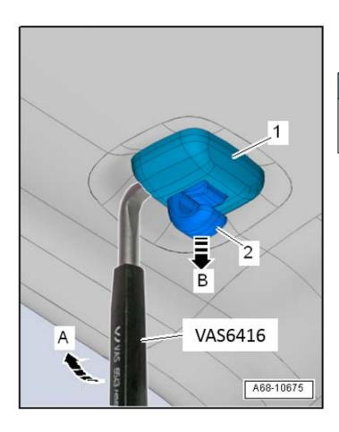
Unclip the sun visor center support cover <1> by sliding the -VAS6416- only about 1 mm under the cap in the direction of <arrow A>.
