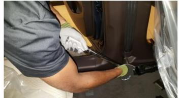
3. Reseat the anchor bolt cover over the anchor bolt and move the driver seat rearward.
