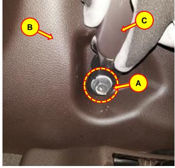
2. Set the torque wrench to nominal (47NM or 34.7 ft-lbs). Apply torque to the anchor bolt until it is tightened to spec.
