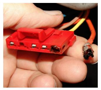
If the female connector to the Blower Motor Resistor assembly exhibits a previous overheat condition, (see photo) replace the harness and resistor assembly with the current replacement parts.
