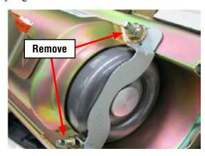
STEP 7- With the stopper plate removed and the other 2 self-locking nuts loosened, unseat the inflator off the mounting bracket end plate then rotate it slightly CLOCKWISE to make it easier to remove as shown in the photo to the right. Slide the inflator out of its mounting while feeding the cut off portion of the wiring harness through the "D-Shaped" hole in the end of the mounting bracket.
