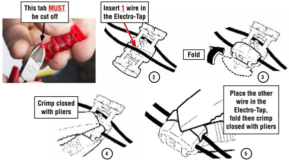
**STEP 5-** Once the Electro-Tap connector is fully crimped in place, cut the 2 wires on the **body harness connector side** of the Electro-Tap connector.
