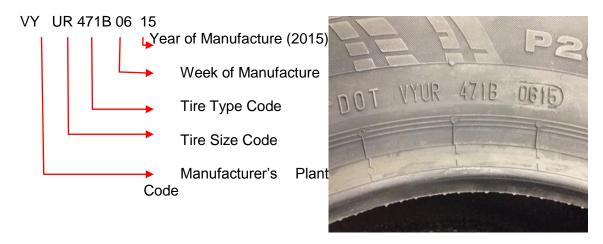
Tires made for use in the United States are required to have the DOT serial number and date located on one sidewall of the tire near the rim. The sample shows a tire manufactured during the 6<sup>th</sup> week of 2015.
