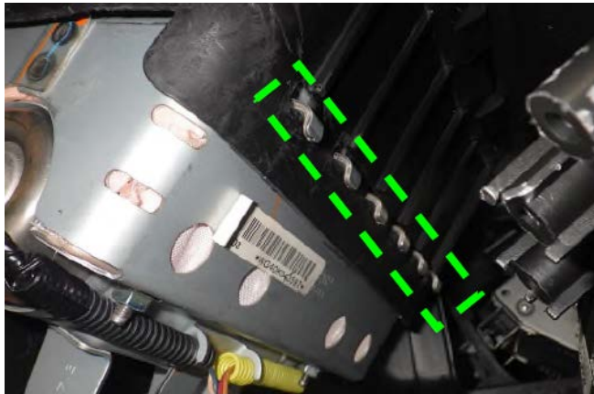
Module in position, retaining claws engaged.
