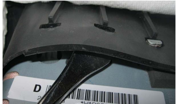
Retaining claws being CAREFULLY disengaged.
