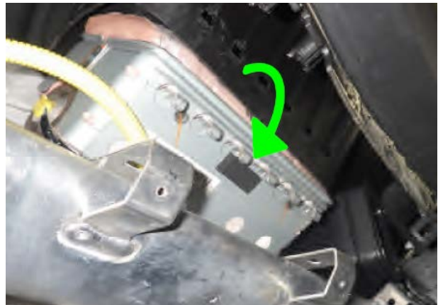
Retaining claws released and module rotated downward to release / remove.
