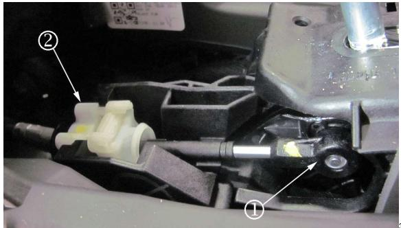
**Note:** Inspect the range selector lever cable at the terminal rod end (1) and bracket end fitting (2). Review steps 3.1-3.2.
