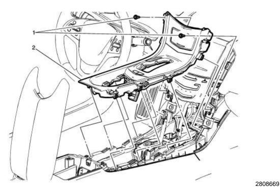
2. Remove the front floor console trim plate (ATS vehicles). Refer to *Front Floor Console Trim Plate Replacement* in SI. Remove the Front Floor Console (CTS vehicles). Refer to *Front Floor Console Replacement* in SI.
