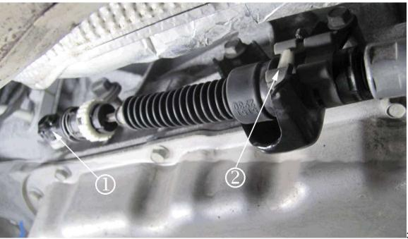
**Note:** Inspect the range selector lever cable at the terminal rod end (1) and bracket end fitting (2). Review steps 5.1-5.2.
