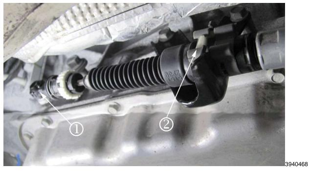
**Note:** Inspect the range selector lever cable at the terminal rod end (1) and bracket end fitting (2). Review steps 5.1-5.2.
