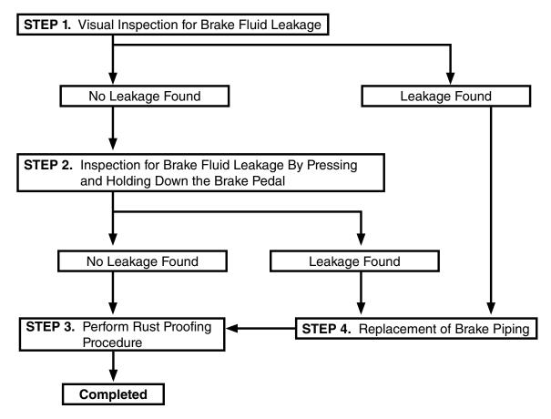
**STEP 1.** Raise the vehicle on a twin-post (symmetrical) lift to perform the inspection of the 4-way connector area of the brake piping for any sign of brake fluid leakage. Open the inspection door located on the right-hand plastic fuel tank cover shown in Photo 1 below. This will provide access to inspect the 4-way connector area of the brake piping which is the focus of this recall.
