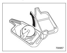
3. Remove the circuit board from the bottom half of the case and remove the batteries.
