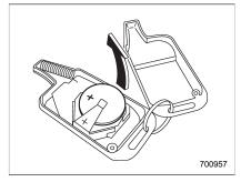
3. Remove the circuit board from the bottom half of the case and remove the batteries.
