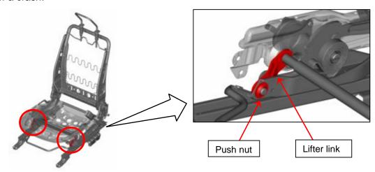
Dealers are instructed to inspect the front lifter links for any crack or damage, and if no crack or damage exists in the lifter links, install reinforcement brackets on the lifter links, and increase the number of push nuts for the rear seat lifter links to two per lifter link.
