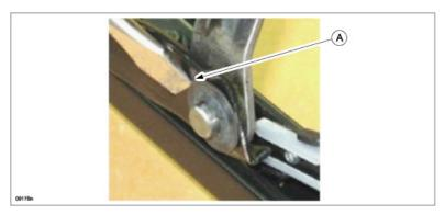
2. Remove the push nut with pliers.
