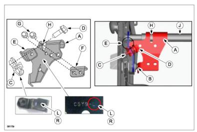
b. At Point (B), attach the side plate to the shaft of the sub slider unit link.
