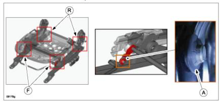
Samples of push nut installed correctly and loose or missing:
