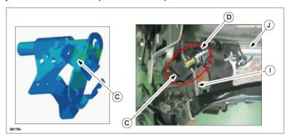
**NOTE:** The side plate (A) and the seat bracket (C) have (R) and (L) stamps for right and left sides. Make sure to install them on the correct side. If the right side and the left side are installed incorrectly, the bracket will interfere with the lifter and will not operate.
