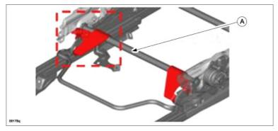
a. Hook the side plate (A) to stabilizer (J). The side plates are stamped with (R) and (L) for right and left sides.
