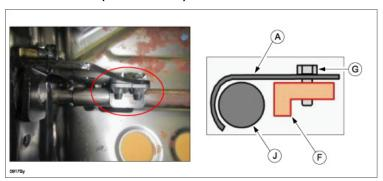
**NOTE:** Mazda2s repaired using TSB 09-043/12 (DRIVER SEAT RATTLE NOISE WHEN STOPPING OR STARTING THE VEHICLE) have a special spring with a long side and short side to reduce seat free play. When mounting the bracket, adjust the spring position so that the long side of the spring can fit in the groove (H) of the bracket on the stabilizer bar.
