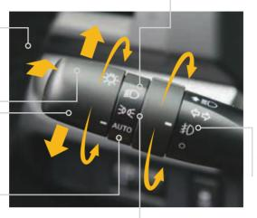
Rotate to turn on fog lights (if equipped).
