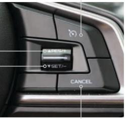
Press the accelerator pedal until your vehicle reaches the desired speed. Push the switch to the "SET" side and release. Ease off the accelerator pedal. Your vehicle will maintain the desired speed.
