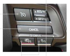
To cancel the cruise control, push the brake pedal or press the "CANCEL" button. If you have a manual transmission, you can push in the clutch pedal.
