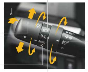
Rotate to turn on fog lights (if equipped).
