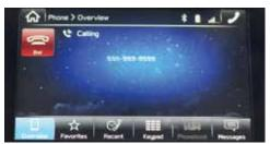
To end the call, press the **PHONE ON HOOK BUTTON** or touch the red "End" soft key.
