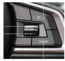
Press the accelerator pedal until your vehicle reaches the desired speed. Push the switch to the "SET" side and release. Ease off the accelerator pedal. Your vehicle will maintain the desired speed. To cancel the cruise control, push the brake pedal or press the "CANCEL" button. If you have a manual transmission, you can push in the clutch pedal.
