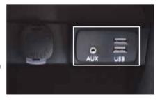
music stored on it through the vehicle speakers. Press the "SOURCE" button located on the audio system to select the auxiliary mode.
