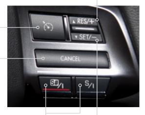
To cancel the cruise control, push the brake pedal or press the "CANCEL" button. If you have a manual transmission, you can push in the clutch pedal.
