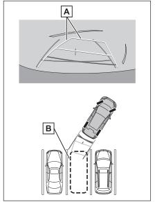
3 When the rear of the vehicle has entered the parking space, turn the steering wheel so that the vehicle width guide lines are within the left and right dividing lines of the parking space.
