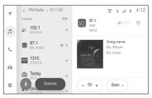
[Scan] : SEEK UP and output the audio of the detected station for 10 sec. This is repeated.
