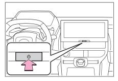
Press and hold the [VOL O] knob for at least 3 seconds.
