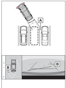
3 When the rear of the vehicle has entered the parking space, turn the steering wheel so that the vehicle width guide lines are within the left and right dividing lines of the parking space.
