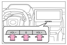
Press [**VOL** O ] knob to turn the audio on and off. Turn the knob to adjust the volume.
