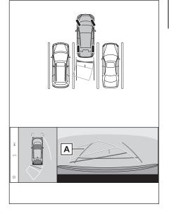
4 Once the vehicle width guide lines and the parking space lines are parallel, straighten the steering wheel and reverse
