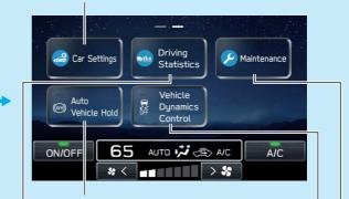
Turn the Auto Vehicle Hold system on/off. Refer to the vehicle Owner's Manual.
