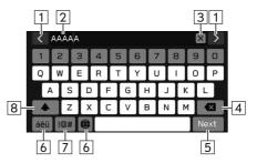
1 Select to move the cursor. Input field 2 • The position of the cursor can be moved by selecting the desired location in the input field. 3 Select to clear the input field. 4 Select to erase one character. 5 Select to enter the item. 6 Select to change keyboard types. 7 Select to enter symbols. 8 Select to enter characters in lower case or in upper case.
