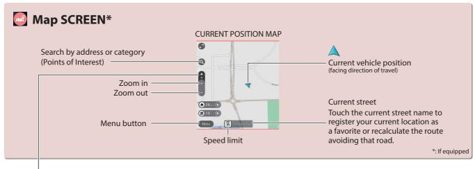
The orientation of the map can be changed between 2D north-up, 2D heading-up and 3D heading-up. P.189
