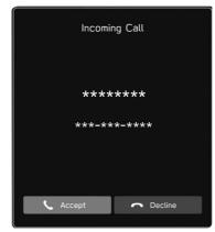
**To refuse to receive the call:** Select **Decline** (Decline) or press the switch on the steering wheel.
