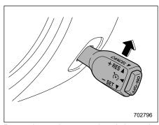
Press the cruise control switch to the "+RES" side and hold it until the vehicle reaches the desired speed. Then, release the switch. The vehicle speed at that moment will be memorized and treated as the new set speed.
