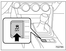
5. Press and hold the Vehicle Stability Control (VSC) OFF switch for 30 seconds until the Vehicle Stability Control (VSC)
