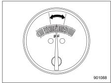
Turn the air compressor switch on and adjust the air pressure to the appropriate level (green zone of the air gauge).
