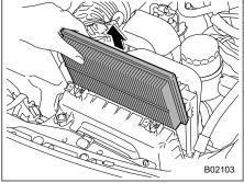
2. Open the air cleaner case and remove the air cleaner element.
