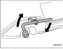
Tighten the towing hook securely using the wheel nut wrench.
