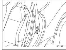
The load capacity of your vehicle is determined by weight, not by available cargo space. The maximum load you can carry in your vehicle is shown on the tire inflation pressure label attached to the driver's side center pillar. It includes the total
