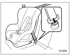
10. To remove the child restraint system, press the release button on the seatbelt
