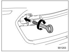
4 Screw the towing hook into the threaded hole until the threads can no longer be seen.
