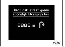
When the route guidance is set in the navigation system, this item shows the navigation route information. For details about the audio system, refer to the separate audio Owner's Manual.
