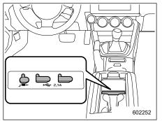
Console USB power supply (an audio device can be connected and used)
