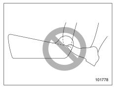
Do not let rear passengers rest their feet between the front seatback and seat cushion. Doing so may interfere with the proper operation of the following systems and could result in serious injury.
