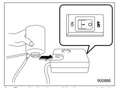
3. Turn the bottle upside down and tilt the bottle cap into the bottle holder of the air compressor.
