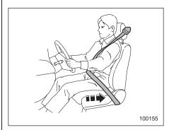
The SRS airbags deploy with considerable speed and force. Occupants who are not seated in proper upright position when the SRS airbag deploys could suffer serious injury. Because the SRS airbag needs enough space for deployment, the driver should always sit upright and back in the seat as far from the steering wheel as practical while still maintaining full vehicle control, and the front passenger should move the seat as far back as possible and sit upright and well back in the seat.
