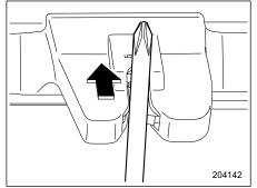
2. To lock it, press the latch with the screwdriver shaft until it clicks.
