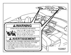
This vehicle has warning labels on the driver's and front passenger's sun visors beginning with the phrase "EVEN WITH ADVANCED AIR BAGS" and a tag attached to the glove box lid beginning with the phrase "Even with Advanced Air Bags". Make sure that you carefully read the instructions on the warning labels and tag.
