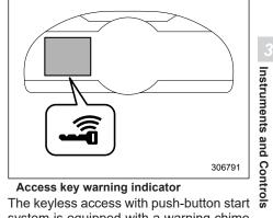
system is equipped with a warning chime and the access key warning indicator in order to minimize improper operations and help protect your vehicle from theft.
