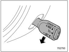
Press the cruise control switch to the "-SFT" side and hold it until the vehicle reaches the desired speed. Then, release the switch. The vehicle speed at that moment will be memorized and treated as the new set speed.
