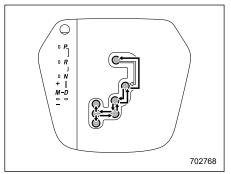
: Shift with the brake pedal depressed and push-button ignition switch in the "ON" position. When shifting between "P" and "D", depress the brake pedal and securely stop the vehicle before shifting.
