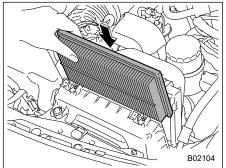
4. Install a new air cleaner element in the way the longitudinal side and the transverse side face as shown in the illustration.
