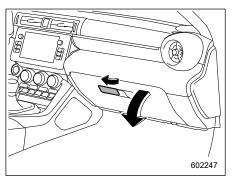
To open the glove box, pull the handle. To close it, push the lid firmly upward.
