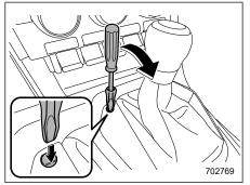
2. Using a flathead screwdriver, remove the cover. To prevent damage to the vehicle, wrap the tip of the flathead screwdriver with a rag, etc.
