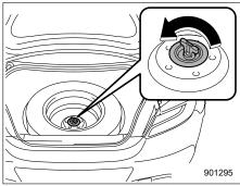
6. Models with spare tire: Take out the under-floor storage compartment and turn the attaching bolt counterclockwise, then take the spare tire out.
