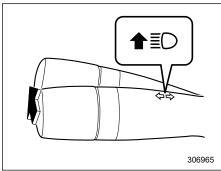
While the light control switch is in the """ or "AUTO" position in a dark place, the headlights will turn on.
