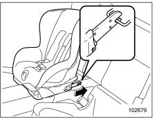
3. While following the instructions supplied by the child restraint system manufacturer, connect the lower hooks onto the lower anchorages located at "when the bottom of the rear seatback. When the hooks are connected, make sure the adjacent seatbelts are not caught.
