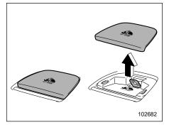
1. Remove the cover flaps to use the anchorages.
