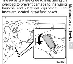
One is located under the instrument panel behind the fuse box cover on the driver's seat side. To remove the cover, pull it out.
