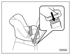
To remove the child restraint system, press the release button on the seatbelt buckle and allow the belt to retract completely. The belt will return to the ELR mode.
