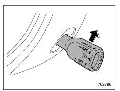
To resume the cruise control after it has been temporarily canceled and with vehicle speed of approximately 20 mph (30 km/h) or more, push the lever up to return to the original cruising speed automatically.
