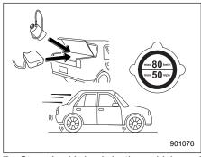
7. Stow the kit back in the vehicle and drive your vehicle immediately for 10 minutes or 3 miles (5 km).
