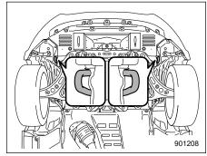
The front tie-down hooks are located between each of the front tires and the front bumper.
