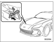
3. Release the secondary hood lock by moving the lever between the front grille and the hood toward the left.
