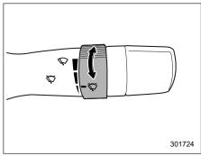
When the wiper switch is in the "\(\nabla\)" position, turn the dial to adjust the operating interval of the wiper. The operating interval can be adjusted in several steps from the shortest interval to the longest.
