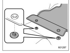
1. Insert the retaining hooks (clips) into the floor mat eyelets.
