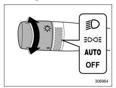
To turn on the headlights, turn the knob on the end of the light control switch.
