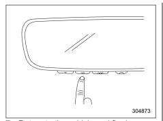
7. Return to the vehicle and firmly press, hold for 2 seconds and release the HomeLink $^{\circledR}$  button up to three times. At this point programming is complete and your device should operate when the HomeLink $^{\circledR}$  button is pressed and released.
