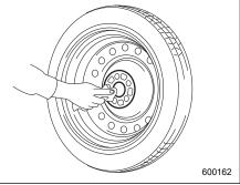
11. Before putting the spare tire on, clean the mounting surface of the wheel and hub with a cloth.
