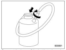
Connect the hose of the bottle to the valve of the bottle in a circular fashion to avoid leakage of the remaining sealant.
