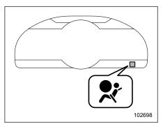
SRS airbag system warning light Have the system inspected by your SUBARU dealer immediately if the SRS airbag system warning light illuminates.
