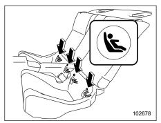
2. You will find "" marks at the bottoms of the rear seatback. These marks indicate the positions of the lower anchorages (bars).
