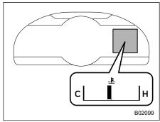
If the radiator cooling fan does not operate even when the engine coolant temperature gauge exceeds the normal operating range, the cooling fan circuit may be defective. Refer to "Engine Coolant Temperature Gauge" P129.
