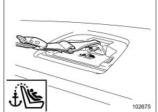
9. Latch the top tether hook onto the tether anchorage that is located behind the rear seat and tighten the top tether firmly. For additional instructions, refer to "Top Tether Anchorages" \$\tilde{F}\$ P58.
