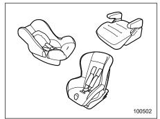
Choose a child restraint system that is appropriate for the child's age and size (weight and height) in order to provide the child with proper protection. The child restraint system should meet all applicable requirements of Federal Motor Vehicle Safety Standards for the United
