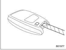
2. Wrap a flat-head screwdriver with vinyl tape or a cloth, and insert it in the gap to remove the cover.
