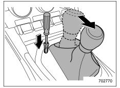
3. While depressing the brake pedal, insert the screwdriver into the hole, press the shift lock release portion using the screwdriver, and then move the select lever.
