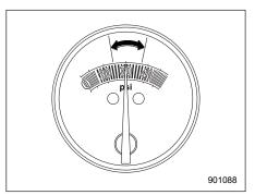
6. Turn the air compressor power switch off when the air pressure reaches the green zone of the air gauge.
