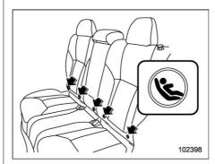
2. There are "©" marks at the bottom of the rear seat seatbacks. These marks indicate the positions of the lower anchorages (bars).
