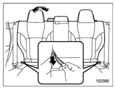
Pull the strap and adjust the seatback to the desired position.
