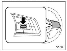
3. Press the "RES/SET" switch to the "SET" side and release it. Then release the
