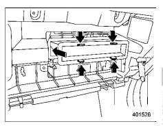
3. Replace the cabin air filter element with a new one.
