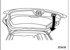
Lower the rear gate slowly and push down firmly until the latch engages.
