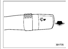
To wash the windshield, pull the wiper control lever toward you. The washer fluid sprays until you release the lever. The wipers operate while you pull the lever.
