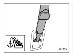
11. Latch the top tether hook onto the tether anchorage that is located behind the rear seat and tighten the top tether firmly. For additional instructions, refer to "Top tether anchorages" #P75.
