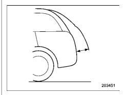
The rear gate cannot be paused when it is in the approximately 2 in (5 cm) range from the fully closed position. The system will ignore any button operation and the rear gate will continue to open.
