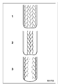
1) Correct tire pressure (tread worn evenly) Roadholding is good, and steering is responsive. Rolling resistance is low, so fuel consumption is also lower.
