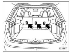
The tether anchorages (upper anchorages) are provided at the locations shown in the above illustration. For details, refer to "Top tether anchorages" \$\tilde{F}\$P75.
