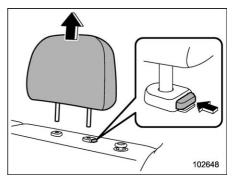
2. Remove the head restraint of the rear seating position where the child restraint system is to be installed. For details, refer to "Head restraints" \$\tilde{F}\$P45.
