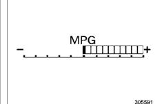
The ECO gauge shows the difference between the current rate of fuel consumption and the average rate of fuel consumption since the trip meter was last reset.
