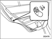
Each rear door has a child safety lock. When the child safety lock lever is in the lock position, the door cannot be opened from the inside. The door can only be opened from the outside.
