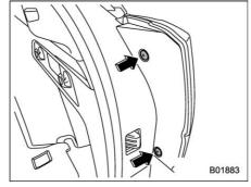
1. Use a screwdriver to remove the secured clips of the covers.
