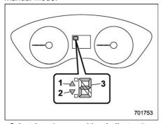
Select lever/gear position indicator (type A)
