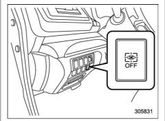
When the Driver Monitoring System OFF switch is pressed, the Driver Monitoring System turns OFF. When the Driver Monitoring System is turned OFF, the Driver Monitoring System OFF indicator on the combination meter display will illuminate. To turn the Driver Monitoring System ON, press the Driver Monitoring System OFF switch again.
