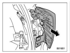
6. Slide the rear combination light assembly rearward to remove it from the vehicle.
