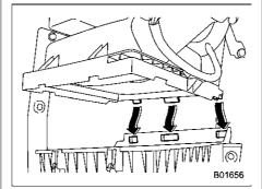
5. To install the air cleaner case (rear), insert the three projections on the air cleaner case (rear) into the slits on the air cleaner case (front).
