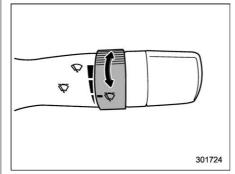
When the wiper switch is in the "T" position, turn the dial to adjust the operating interval of the wiper. The operating interval can be adjusted in several steps from the shortest interval to the longest.
