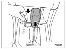
3. While depressing the brake pedal, insert a screwdriver into the hole, press the shift lock release button using a screwdriver, and then move the select lever.
