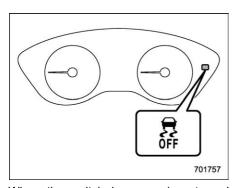
When the switch is pressed or turned during engine operation, the Vehicle Dynamics Control OFF indicator light "8" on the combination meter illuminates. The Vehicle Dynamics Control system will be deactivated and the vehicle will behave like a model not equipped with the Vehicle Dynamics Control system. When the switch is pressed again (type A) or turned to the "NORMAL" side (type B) to reactivate the Vehicle Dynamics Control system, the Vehicle Dynamics Control OFF indicator light turns off.
