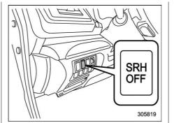
You can turn the SRH function on or off by pressing the SRH OFF switch.
