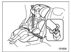
6. To remove the booster seat, press the release button on the seatbelt buckle and allow the belt to retract.
