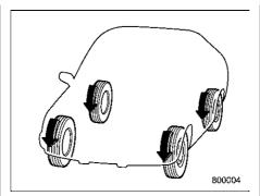
All-Wheel Drive distributes the engine power to all four wheels. AWD models provide better traction when driving on slipperv, wet or snow-covered roads and when moving out of mud, dirt and sand. By shifting power between the front and rear wheels, SUBARU AWD can also provide added traction during acceleration and added engine braking force during deceleration.
