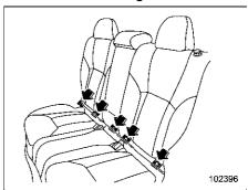
There are a total of 5 lower anchorages at the rear seat. The rear anchorage from the right side is used for both the right seat and center seat. Each lower anchorage is located where the seat cushion meets the seatback
