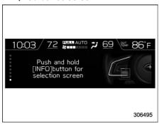
When the INFO button on the steering wheel is pressed and held on this screen, the setting screen can be displayed. For details, refer to "Setting screen" P218.
