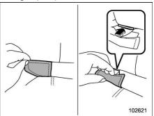
Peel off the anchorage cover from the selected side of the rear seatback. Fold the peeled anchorage cover in half and affix it with hook and loop tape to expose the anchorages (bars) to be used for installation of the child restraint system.
