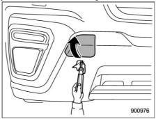
2. Cover the tip of a flat-head screwdriver with vinyl tape or cloth so that it will not
