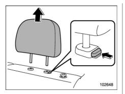
4. Remove the rear seat head restraint. For details, refer to "Head restraints" \$\textit{\$^{\textit{P}}\$P45.}\$
