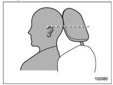
Each head restraint should be adjusted so that the center is closest to the top of the occupant's ears.
