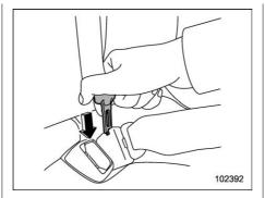
2. Insert a tongue plate or other hard pointed object into the slot in the anchor buckle on the right-hand side and push it in. The anchor tongue plate will then disconnect from the buckle.
