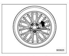
8. Loosen the wheel nuts using the wheel nut wrench but do not remove the nuts.
