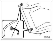
Retaining pins are located on the driver's side floor.
