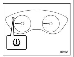
The tire pressure monitoring system provides the driver with a warning message when tire pressure is severely low.
