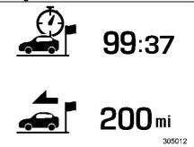
This screen displays the journey time (the time that has elapsed since the ignition switch was turned to the "ON" position) and journey distance (the distance that has been driven since the ignition switch was turned to the "ON" position).
