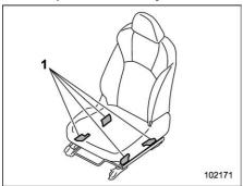
1) Occupant detection system sensors
