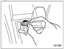
2. Wrap the tip of a flat-head screwdriver
