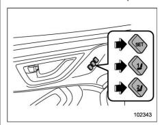
2. Press and hold the "SET" button, then press button "1" or "2" to register the seat position and outside mirror angle.
