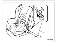
5. Run the lap and shoulder belt through or around the child restraint system following the instructions provided by its manufacturer.
