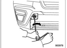
4. Tighten the towing hook securely using
