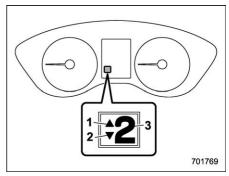
Select lever/gear position indicator (type B)
