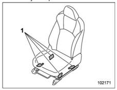
1) Occupant detection system sensors
