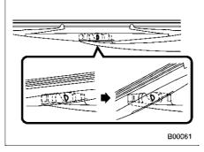
2. Turn the wiper blade assembly counterclockwise.
