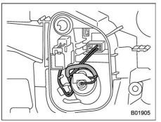
6. Install the light cover on the rear gate.
