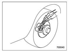
The disc brake pad wear warning indicators on the disc brakes give a warning noise when the brake pads are worn.
