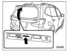
1. Keep pressing the rear gate opener button until it is unlocked (for approximately 5 seconds) and lift up the rear gate.
