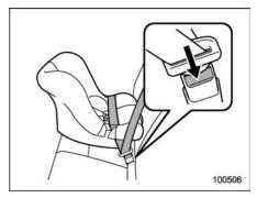
9. To remove the child restraint system, press the release button on the seatbelt buckle and allow the belt to retract completely. The belt will return to the FIR mode.
