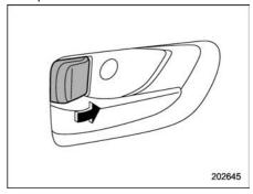
2. Rotate the lock lever forward.
