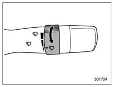
When the wiper switch is in the "\overline{\to}" position, turn the dial to adjust the operating interval of the wiper. You can adjust the operating interval in several steps.
