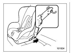
4. While following the instructions supplied by the child restraint system manufacturer, connect the lower hooks onto the lower anchorages located at "@" marks on the bottom of the rear seatback. When the hooks are connected, make sure the adjacent seatbelts are not caught.
