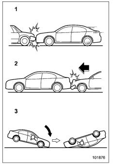
The vehicle is involved in frontal collision with another vehicle (moving or station-
