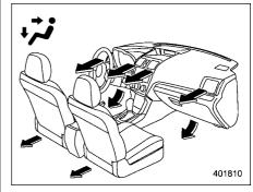
(Bi-level): Instrument panel outlets and foot outlets
