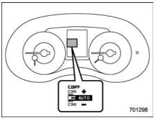
In the auto mode, the system estimates the driving and road conditions using signals from the wheel speed sensor, throttle position sensor, steering angle sensor and brake switch, etc. According to the result, it electronically and automatically controls the degree of limitation of the differential action (LSD torque) to optimize the differential action of the center differential. When you turn the ignition switch ON, the "AUTO" indicator on the combination meter appears.
