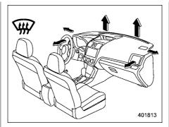
**(Defrost):** Windshield defroster outlets and both side outlets of the instrument panel (Refer to "Defrosting" \$\sigma 4-9.)
