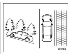
When parking on a hill, always turn the steering wheel. When the vehicle is headed up the hill, turn the front wheels away from the curb.
