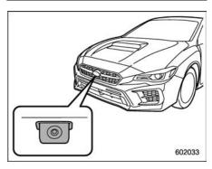
The image from the camera mounted inside the front grille is displayed in the multi-function display (color LCD). This eliminates blind spots and allows the driver to check the forward direction of both sides
