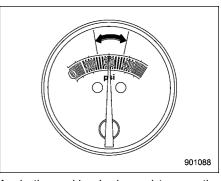
Apply the parking brake and turn on the ignition switch to the "ACC" position. Turn the air compressor switch on and adjust the air pressure to the appropriate level (green zone of the air gauge).
