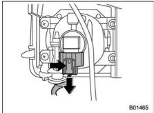
3. Disconnect the electrical connector from the bulb as pushing the tab.
