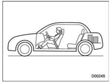
Vehicle capacity weight of the vehicle is 900 lbs (408 kg), which is indicated on the vehicle placard with the statement "The combined weight of occupants and cargo should never exceed 900 lbs or 408 kg".
