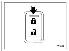
6. Press the front side ("LOCK" side) of the power door locking switch to set the door locks.
