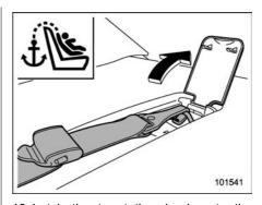
10. Latch the top tether hook onto the tether anchorage that is located behind the rear seat and tighten the top tether firmly. For additional instructions, refer to "Top tether anchorages" \$\tilde{T}\$ 1-33.
