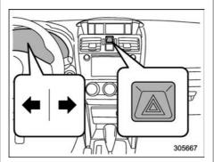
Use the hazard warning flasher to warn other drivers when you have to park your vehicle under emergency conditions. The hazard warning flasher works regardless of the position of the ignition switch.
