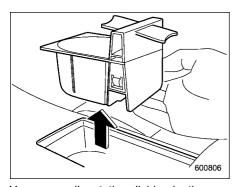
You can pull out the divider in the cup holder and insert it in a different position (further toward the front or rear) to enable cups of different sizes to be held.
