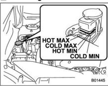
The power steering fluid expands greatly as its temperature rises; the fluid level differs according to fluid temperature. Therefore, the reservoir tank has two different checking ranges for hot and cold fluids.
