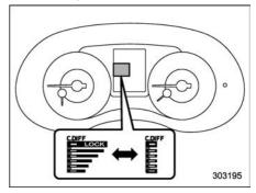
All the indicators will flash when the driver's control center differential has a malfunction. Have the vehicle inspected by your SUBARU dealer. For details, refer to "Driver's Control Center Differential (C. DIFF/DCCD) (STI)" \$\textit{\$\textit{#}}7-19.
