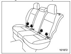
The lower anchorages (bars) are used for installing a child restraint system only in the rear seat window-side seating positions. For each window-side seating position, two lower anchorages are provided. Each lower anchorage is located behind the cover of the seatback bottom.
