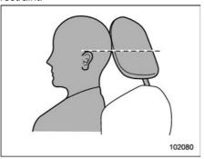
Adjust each head restraint so that the center of the head restraint is closest to the top of the occupant's ears.
