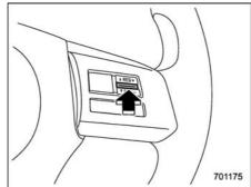
Press the "RFS/SFT" switch to the "RFS" side and hold it until the vehicle reaches the desired speed. Then, release the switch. The vehicle speed at that moment will be memorized and treated as the new set speed.
