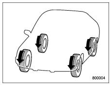
All-Wheel Drive distributes the engine power to all four wheels. AWD models provide better traction when driving on slipperv, wet or snow-covered roads and when moving out of mud, dirt and sand. By shifting power between the front and rear wheels, SUBARU AWD can also provide added traction during acceleration and added engine braking force during deceleration.
