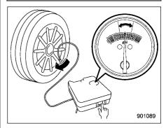
8. After driving for 10 minutes or 3 miles (5 km), whichever comes first, stop the vehicle in a safe place to recheck the air pressure (see step 4).
