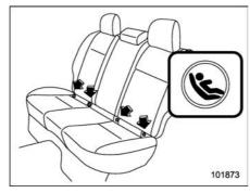
2. You will find marks "Q" at the bottom of the rear seat seatbacks. These marks indicate the positions of the lower anchorages (bars).
