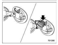
3. Set the fuel filler cap on the cap holder inside the fuel filler lid.
