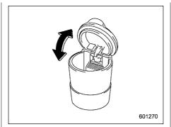
You can install the portable ashtray in each cup holder or bottle holder. For the locations of the cup holders, refer to "Cup holders" @6-6. For the locations of the bottle holders, refer to "Bottle holders" @ 6-7.
