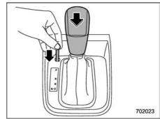
4. While depressing the brake pedal, insert a screwdriver into the hole, press the shift lock release button using a screwdriver, and then move the select
