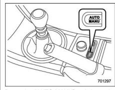
Press the "AUTO-MANU" switch on the center console to switch from auto mode to manual mode or vice versa. When you select the auto mode, the "AUTO" indicator appears. When you select the manual mode, the "AUTO" indicator disappears.
