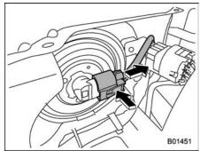
2. Disconnect the electrical connector from the bulb as pushing the tab.
