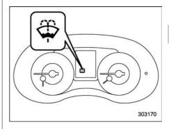
The windshield washer fluid warning indicator appears when the washer fluid level in the tank has dropped to the lower limit. If the warning indicator appears, refill the tank with fluid. For the refilling procedure, refer to "Windshield washer fluid" @ 11-38.
