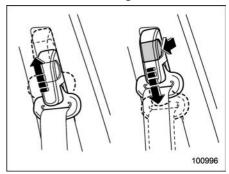
Adjust the shoulder belt anchor height to the position best suited for the driver/front passenger. Always adjust the anchor height so that the shoulder belt passes over the middle of the shoulder without touching the neck.
