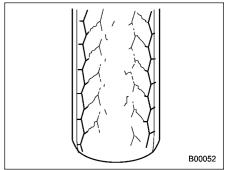
Ride comfort is poor. Also, the tire magnifies the effects of road-surface bumps and dips, possibly resulting in vehicle damage.
