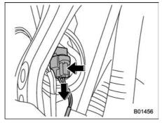
1. Disconnect the electrical connector from the bulb as pushing the tab.
