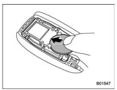
4. Insert a new battery with its positive (+) side facing upward as shown in the figure.
