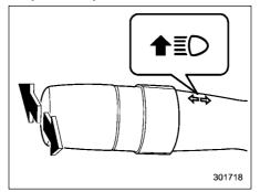
To change from low beam to high beam, push the turn signal lever forward. When the headlights are on high beam, the high beam indicator light "=" on the combination meter is also on.
