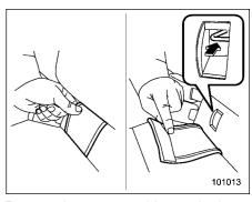
Remove the covers and locate the lower anchorages (bars).
