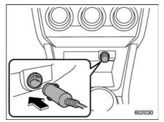
4. Connect the power plug of the air compressor into the accessory power outlet.
