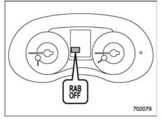
Reverse Automatic Braking system OFF indicator
