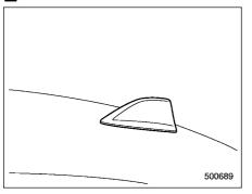
The shark-fin type roof antenna is installed in the center at the rear of the roof.
