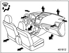
(Heat-def): Windshield defroster outlets, foot outlets and both side outlets of the instrument panel (Refer to "Defrosting" \$\tilde{\pi} 4-9.)\$
