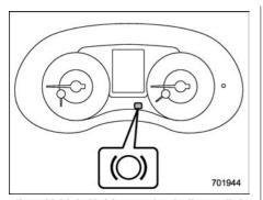
Auto Vehicle Hold operation indicator light While the vehicle is kept stopped by the Auto Vehicle Hold function, the Auto Vehicle Hold operation indicator light will illuminate.
