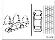
When facing downhill, turn the front wheels into the curb.
