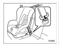
11. To remove the child restraint system, press the release button on the seatbelt buckle and allow the belt to retract completely. The belt will return to the FIR mode.
