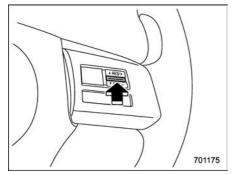
To resume the cruise control after it has been temporarily canceled and with vehicle speed of approximately 20 mph (30 km/h) or more, press the "RES/SET" switch to the "RES" side to return to the original cruising speed automatically.
