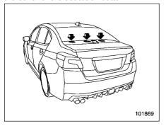
The tether anchorages (upper anchorages) are provided at the locations shown in the above illustration. For details. refer to "Top tether anchorages" \$\alpha\$1-33.
