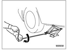
9. Insert the jack handle into the jackscrew, and turn the handle until the tire clears the ground. Do not raise the vehicle higher than necessary. 10. Remove the wheel nuts and the flat tire.
