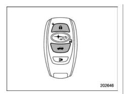
3. Press and hold the "A" button and " button on the access key fob simultaneously for more than 5 seconds.
