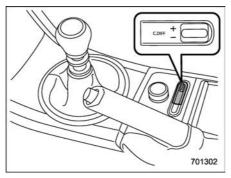
The control switch is located beside the parking brake lever. Push the control switch forward or pull it rearward to change the initial LSD torque.
