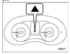
When the Intelligent (I) mode is selected, a shift-up indicator "\( \Lambda \)" on the combination meter will blink to signal the best time to shift gears for maximum fuel efficiency.
