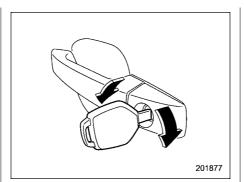
To lock the driver's door from the outside with the key, turn the key toward the front. To unlock the door, turn the key toward the rear. Pull the outside door handle to open an unlocked door.
