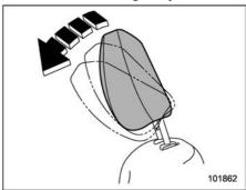
It is possible to adjust the angle of the head restraint in several steps. While maintaining a suitable driving posture, adjust the head restraint to a position where the back of your head is as close to the head restraint as possible.
