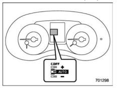
This indicator functions while the ignition switch is "ON". When it appears, it indicates that the driver's control center differential is set to the auto mode. It disappears when the driver's control center differential is set to the manual mode. For details, refer to "Driver's Control Center Differential (C.DIFF/DCCD) (STI)" \$\infty 7-19\$.
