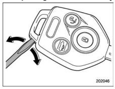
Open the key head using a flat-head screwdriver.
