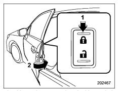
Locking using power door locking switch
