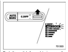
Push the switch forward to increase the initial LSD torque; when the "LOCK" indicator appears, the initial LSD torque setting is maximum. The center differential will then be almost completely locked.
