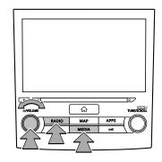
"<sup>(b</sup>/VOLUME" knob: Press and hold to turn the audio system off, and press to turn it on again. The system turns on in the last mode used. Turn this knob to adjust the volume. Press to mute the audio system.
