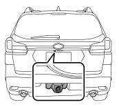
When the ignition switch is "ON" and the select lever is set to "R", the rear view camera automatically displays the rear view image behind the vehicle. The rear view camera image is displayed on this system.
