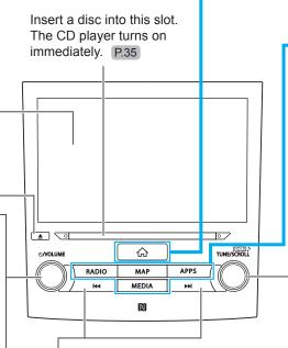
Press button to seek up or down for a radio station or to access a desired track/file. Press and hold button to fast forward/ rewind files or tracks.
